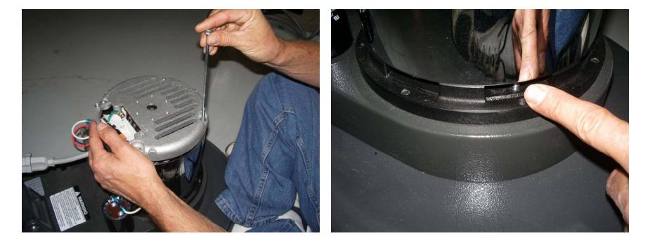
Insert the four bolts that hold the motor top casting to the motor base.
