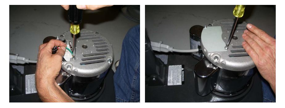
Once the motor top casting is secured in place reconnect the ground wire. DO NOT OPERATE THE EQUIPMENT WITHOUT THE GROUND WIRE CONNECTED.
