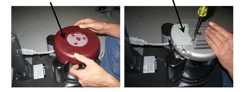
Remove motor cover (195004) and set aside for reassembly
