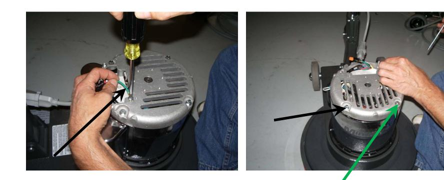
Remove the screw holding the green ground wire to motor, set aside for re-assembly.
