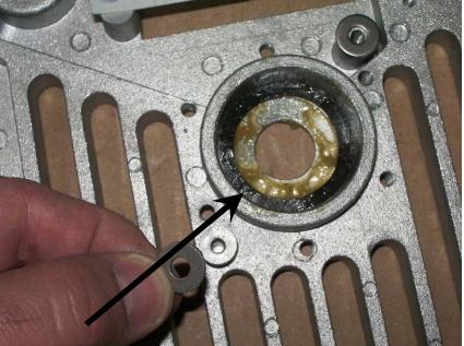
Place the two washers (712764) on the start switch stand offs. One washer is required on each standoff.
