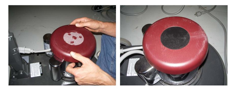
Put the motor cover back in place and attach with screws.
