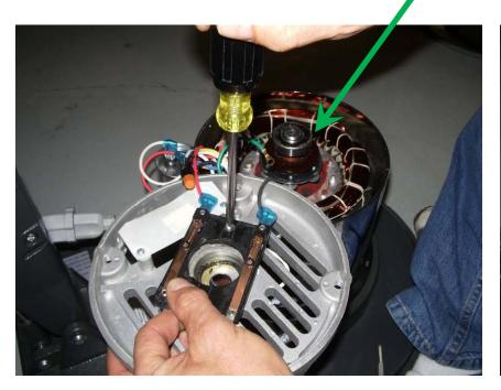
Put the start switch back in place and tighten down the mounting screws. Do not over tighten the mounting screws.
