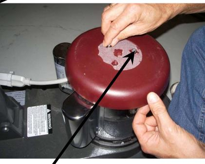
Remove the decal (715459) that covers the motor cover screws 999136 REV \* 11/10 JP
