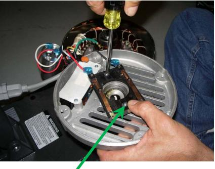
Remove the motor top casting and fold back for access to the start switch. Note: It may be necessary to <u>tap</u> on the casting with a rubber mallet to remove it. Use caution so there is no damage to the internal components.
